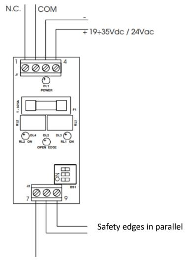
Connect to the failsafe test terminal on the FAAC gate control board
