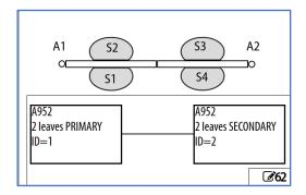
If you are installing the operators on a double door, you will need to enable the Primary /Secondary functionality of the 952. In order to do this, you will require the use of a KP EVO (Part Number: 790022) as it is NOT POSSIBLE to achieve this otherwise. Please note that the A952 can only be configured as Primary /Secondary with another 952 of the same firmware/software versions.
