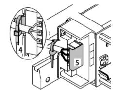
Install the terminal board plastic protective cover. Power on.
