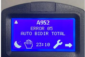
Error 5 will be displayed for 30 seconds, or a reset can be carried out.
