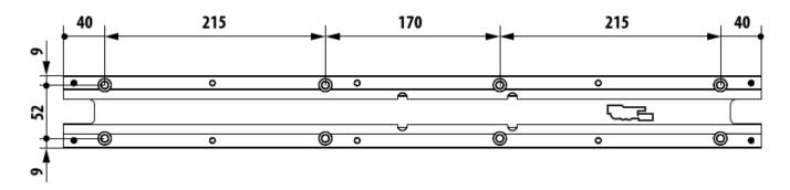
Use appropriate fixings for the material that you are fixing the operator to. In General, 60mm of Softwood, 40mm of Hardwood, 6/10mm of Aluminium or 6mm of Steel are suitable mounting requirements.
