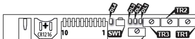
Please note that if the KP EVO is used for Programming, DL4 will illuminate "YELLOW" but **DO NOT** press SW1 as this will revert back to DIPSWITCH or TRIMMER setting.
