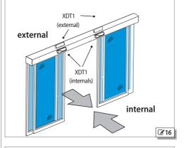
Dual technology radar/infrared detector connection
