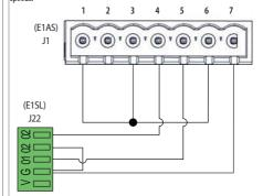
Example 2: connection of AIRSLIDE inputs for operating at 1 speed.
