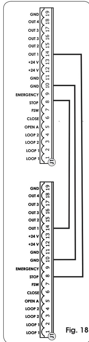
For in-line barriers, enable OUT1 INTERLOCK on parameter 18 (see 2nd PROGRAMMING LEVEL) on both boards and connect them as shown in fig. 18
