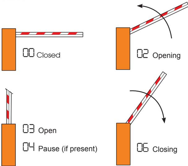
In the sequence, states 01 and 05 are not shown; these correspond to pre-flashing at opening and at closing, respectively.
